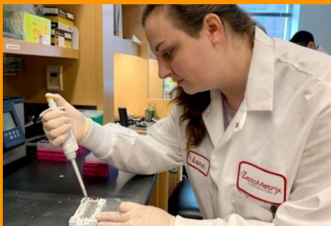
ZeptoMetrix molecular biologist Lauren Morrow loads reagents into a cartridge used in a digital droplet PCR platform with an automated droplet generator. Photo: Karuna Sharma.
